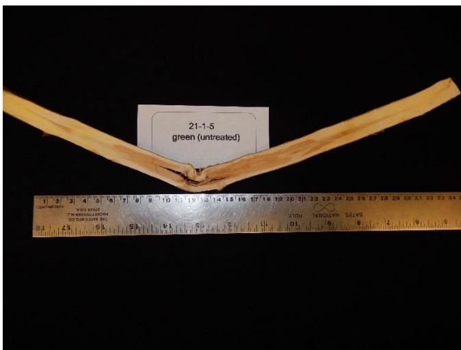
stain. In this case, the fungus caused the branch to weaken and break.
