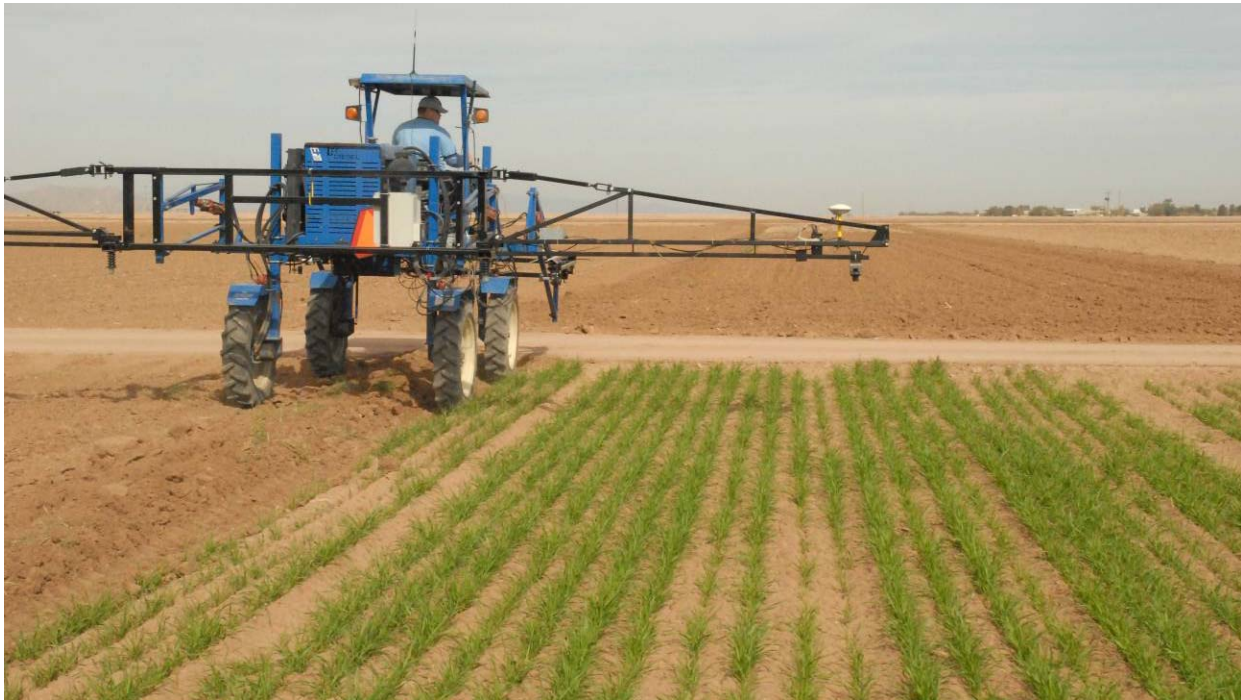
Figure 2. Field deployment of sensors in mobile platform. System set up in boom to continuously collect canopy spectral data.
