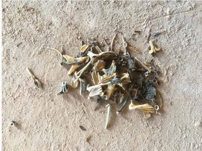
Figure 1. Fish bones found in the pipe leading to the pump.
