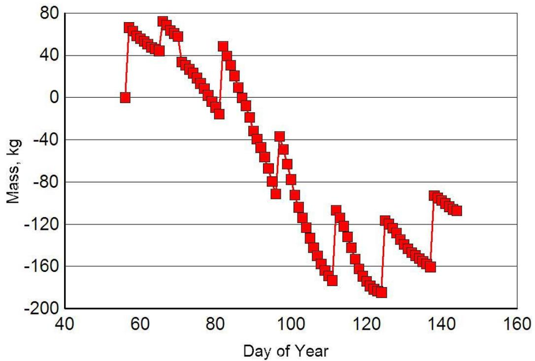
Figure 8. Calculated water balance in lysimeter 4 in 2010.
