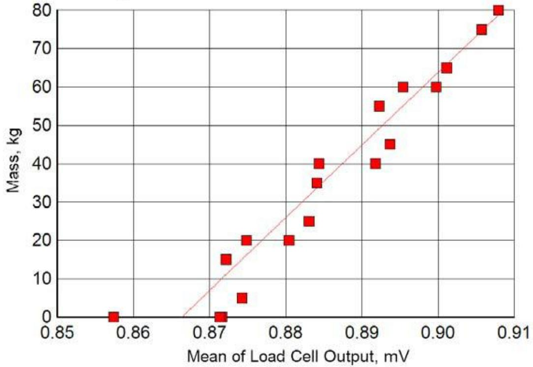
Figure 2. Calibration line of load cell output (mV) and mass (kg) for lysimeter #2.
