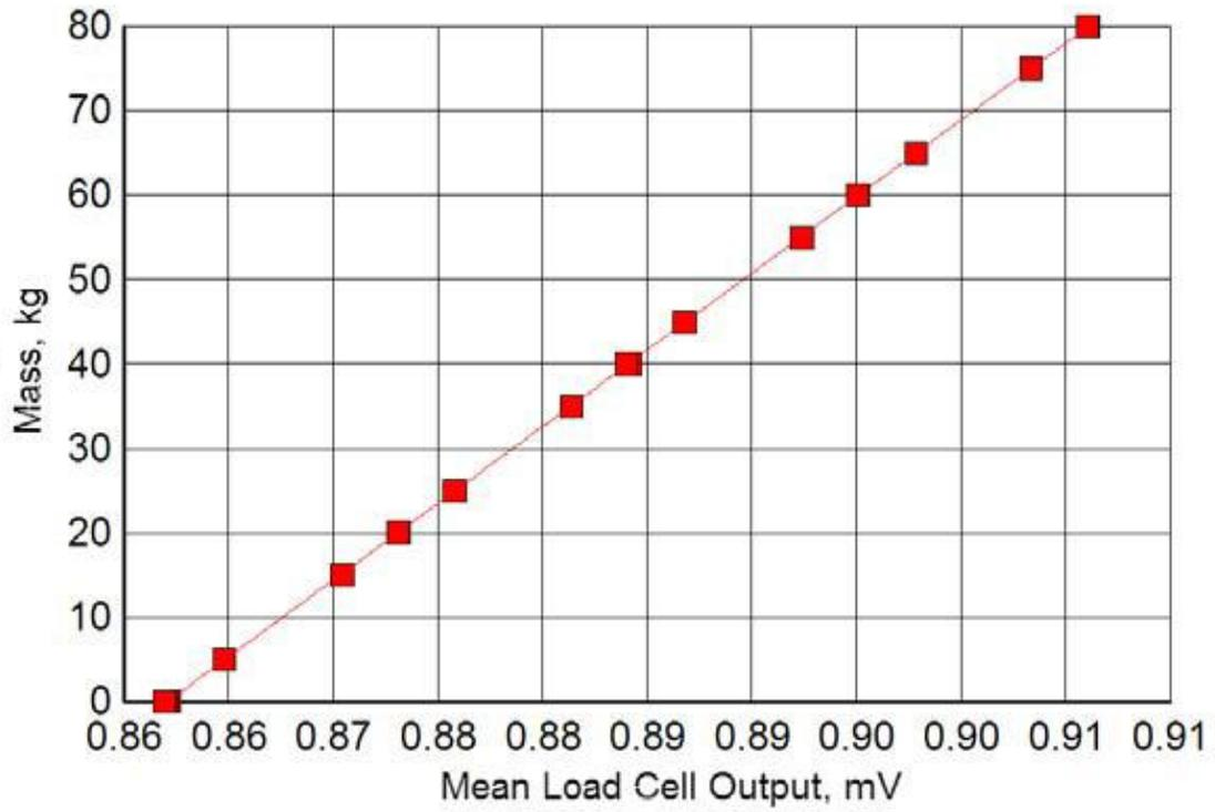
Figure 3. Calibration line of load cell output (mV) and mass (kg) for lysimeter #3.
