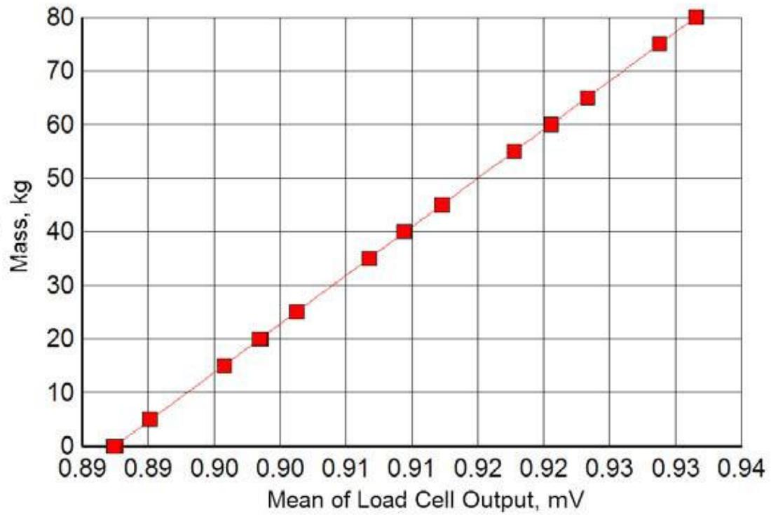
Figure 4. Calibration line of load cell output (mV) and mass (kg) for lysimeter #4.
