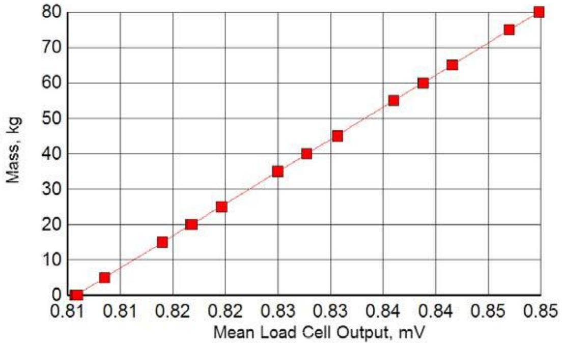
Figure 1. Calibration line of load cell output (mV) and mass (kg) for lysimeter #1.
