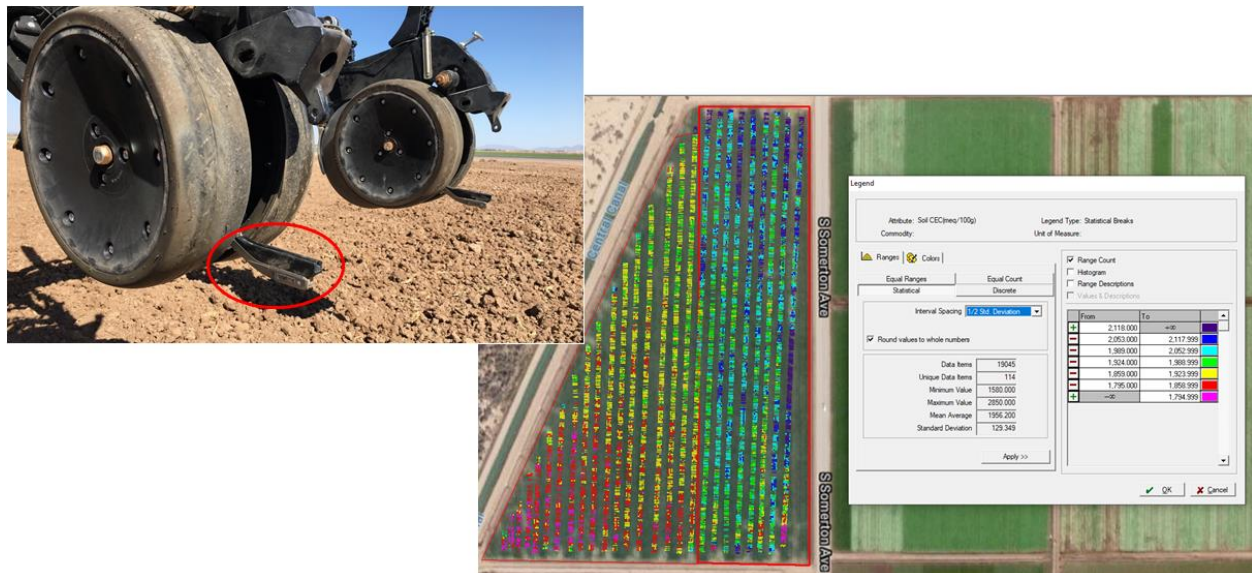
Figure 1. Picture of soil spectroscopy sensor (upper left) deployed in a commercial field during soil preparation. Map on the right side shows the distribution of soil CEC values in the field under study.
