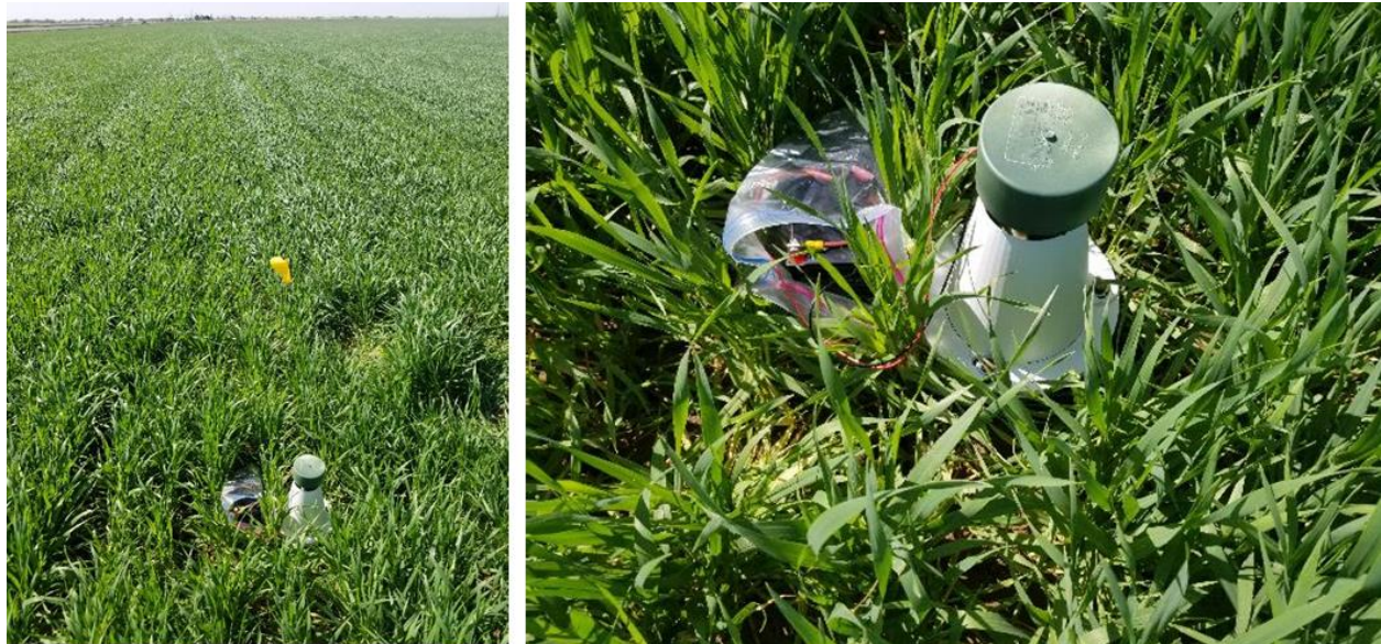
Figure 2. Left picture: Field deployment of low-cost soil respiration sensor in a durum wheat field in Somerton AZ. Right picture: Close view of sensor installed for continuous measurement of CO 2 released at the soil surface due to below-ground microbial and crop root activity.
