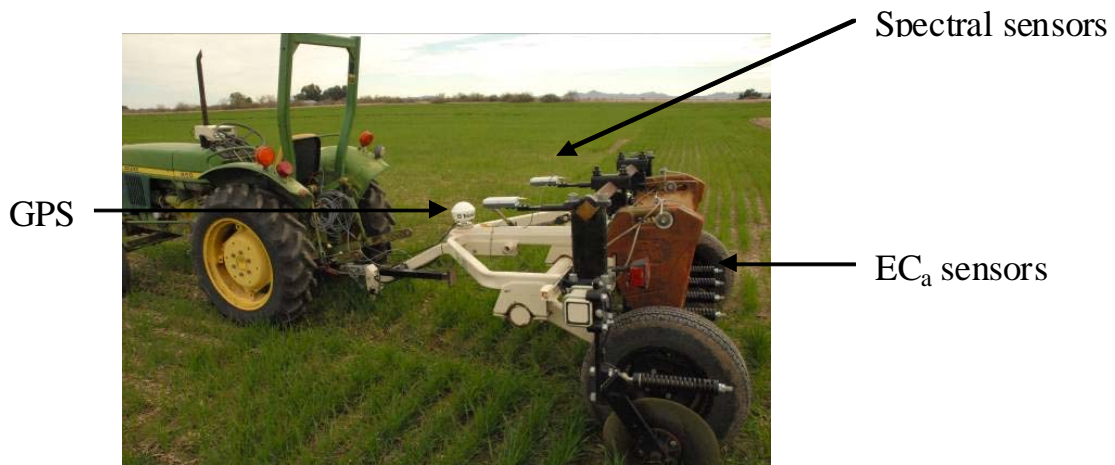
Figure 1. Field deployment of EC and spectral sensors in Sacaton AZ. January 2010
