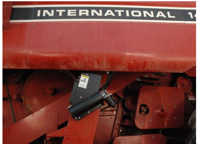
Figure 2. Grain mass flow sensor (left) and moisture sensor (right) installed in grain combine for yield monitoring operations. Maricopa Agricultural Center – May 2010
