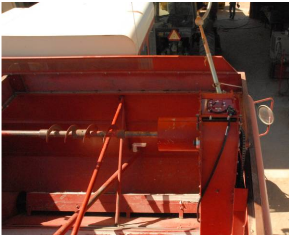
Figure 2. Grain mass flow sensor (left) and moisture sensor (right) installed in grain combine for yield monitoring operations. Maricopa Agricultural Center – May 2010
