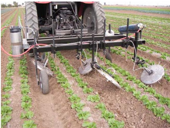
**Figure 2. Spike wheel fertilizer applicator configured to inject liquid chemicals into sidewalls of lettuce beds.**
