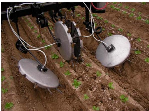
**Figure 3. Spike wheel fertilizer applicator configured to inject liquid chemicals into sidewalls and top of lettuce beds.**
