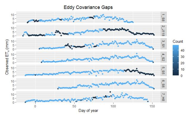
Figure 2. Eddy covariance daily data gap. Observed daily ET<sub>c</sub> from the seven sites are shown by their corresponding day of year. Daily observations with no gaps, 48 samples (from 30-minute time averages) are coded blue. Observations with gaps are coded with progressively darker gray values as the valid sample counts decrease. S2, S6, and H8 sites had the fewest gaps, while J118 had the greatest. S5 was mostly gap-free except for the final 30 days of the 2018 experiment.
