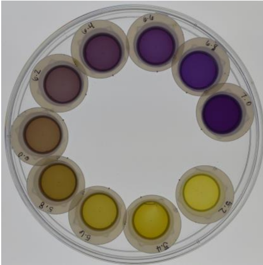
Figure 2. Reference pH colors used in rhizosphere acidification screening.
