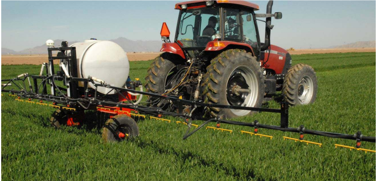
Figure 2. Ground system to apply liquid fertilizer in experimental plots in Maricopa AZ on March 4, 2011. System utilized electronic section and flow control to deliver accurate application rates.
